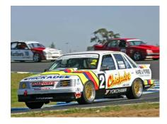
All of the above cars as well as a few others are "set-up" by Sonic, we scale the cars ie the cars are placed on 4 x scales that are set dead level using a laser. The cars ride heights, cambers, toes, castors etc are all trimmed & each wheels weight is set for what I believe is the best for that given car/driver/track combination. This set-up usually changes from track to track due to differing speeds, directions, bumps & aerodynamics etc.
